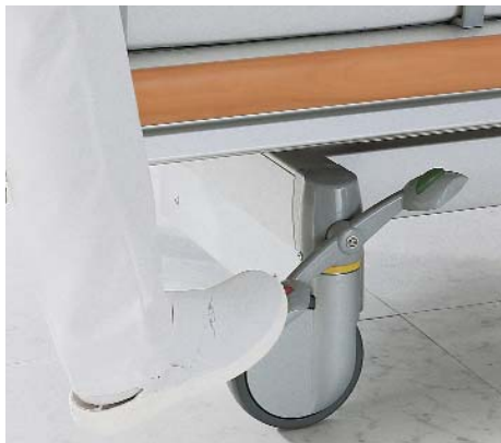
Left figure: Series S 380 and S 280 healthcare beds are equipped with easy to roll casters that can be centrally locked by a foot brake lever. Full swivel function and straight steering can also be achieved with the foot lever. Shown with (optional) closed caster.
